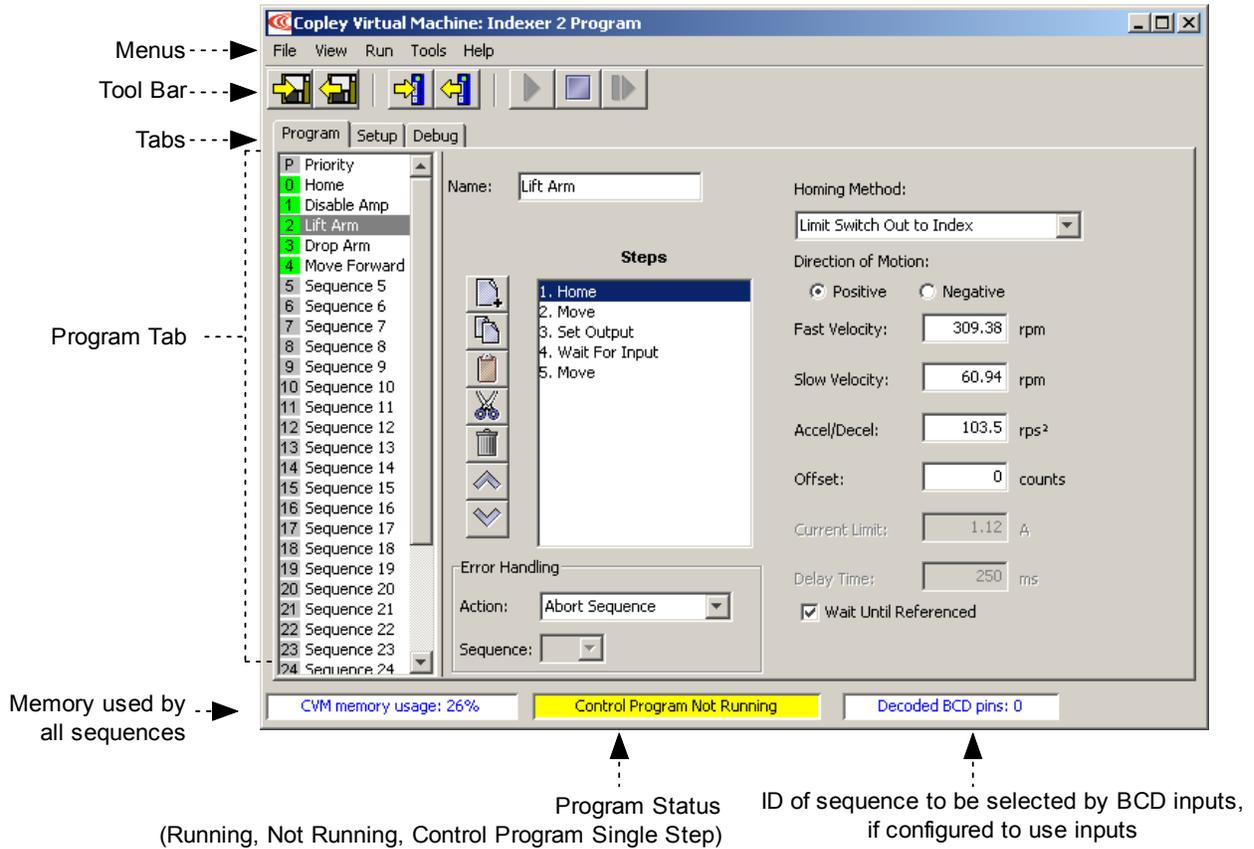
The *Program* tab is used to create and modify sequences.
