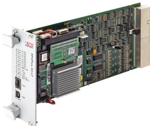
The SPiiPlusNT (NT - Network Controller) is designed for incorporation in the MC4U. Once plugged into an MC4U, the MC4U becomes also an EtherCAT master designated MC4U<sub>nt</sub>. It manages the EtherCAT network with up to 32 axes of motion and countless number of I/Os and sensor modules. The SPiiPlusNT also includes Servo Processors for controlling local drives that reside within the same MC4U<sub>nt</sub> enclosure.
