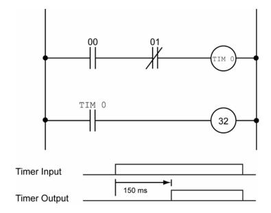
The following PLC code fragment implements the ladder logic shown above. Lines 100 and 110 create a new logic block. Line 120 connects the block to timer 0 and sets the timer to 150 milliseconds. Lines 130 and 140 connect the timer output to relay 32.
