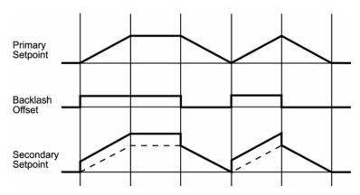
**NOTE:** The primary setpoint is the summation of the current position and the total cam, gear, and jog offsets. The secondary setpoint is the summation of the primary setpoint and the total ballscrew and backlash offsets. The secondary setpoint is the one that is actually used by the servo loop.
