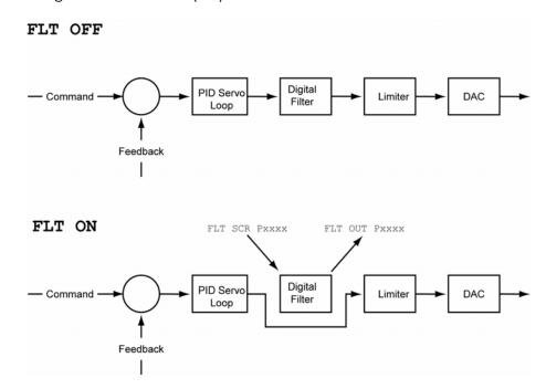
**NOTE:** This filter is still updated in the servo loop block. The sequence in which the input, output and digital filter will update should be carefully sought, so that nothing is overwritten.
