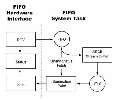
The ACR9000 controller differs—it has COM1, COM2, and STREAM1 through STREAM5. The controller can manage up to five connections, in any combination of ASCII or Ethernet/IP. There are five communication streams for connection, with STREAM1 dedicated to USB.
