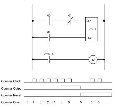
The following PLC code fragment implements the ladder logic as shown in the illustration above. Lines 100 and 110 create the first block. Line 120 creates the second block. Line 130 connects the two blocks to counter 1 and sets the count to 5. Lines 140 and 150 connect the counter output to relay 32.
