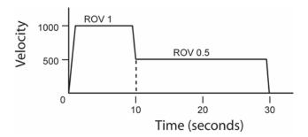
ROV 1 : REM ensures is set to default DEC 1000 ACC 1000 STP 1000 VEL 1000  $\rm X/20000$  : REM incremental move DWL 10 : REM dwell for ten seconds
