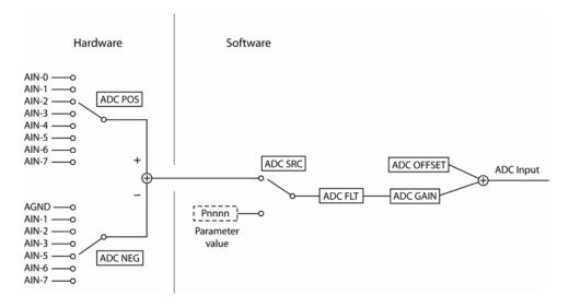
Parameter value in the above drawing is any system parameter (P4096 and up). The switch at ADC SRC is in the NONE position (using onboard ADCs).
