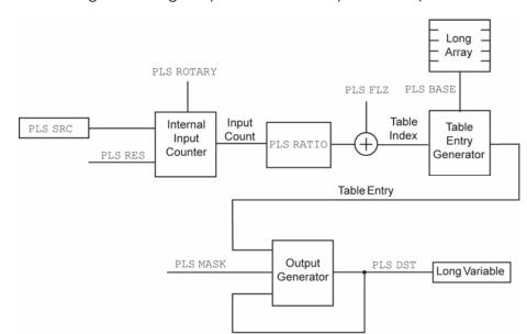
The following block diagram provides an example of PLS operation:
